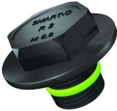
Once in contact with motor oil and heat, the o-ring expands up to 20 percent creating a seal between the opposing threads. This produces a positive connection between the drain plug and the oil pan, allowing the oil pan and plug to vibrate at the same frequency.
