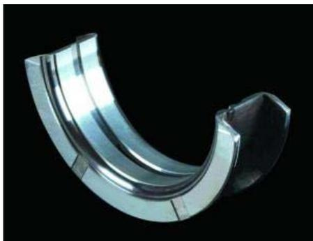
King bearings feature the closest wall tolerances in the industry (Bull's Eye Tolerance), with all shells matched to .0001 inch. Main and rod bearings are narrowed for large radii crankshafts. In addition to main and rod bearings, King also offers camshaft bearings and thrust washers.
