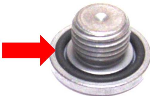
Example of oil drain plug requiring low torque to be applied.
